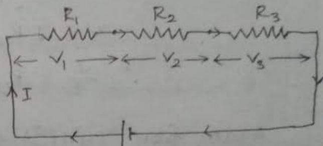
Let,  $I$  is the current flowing through each resistor and  $V_1$ ,  $V_2$  &  $V_3$  be the potential differences across  $R_1$ ,  $R_2$  &  $R_3$  respectively.
