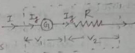
Let,  $I_g$  is the current through galvanometer of resistance  $G$  and  $R$  is the very high resistance. Then,
